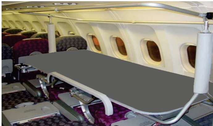
Picture 1. Replacement of passenger seats to medical stretchers in the cabin of aircraft
