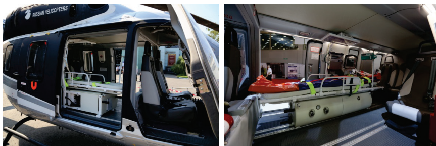
Picture 2. Medical equipment of an "Ansats" helicopter
